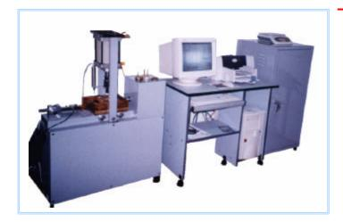
Computer-controlled pneumatic loading system. Pressurize weight is not required.
